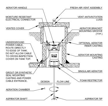
Each Singulair aerator is a precision engineered electro-mechanical device. Do not remove it from its installed position. Do not attempt any type of repair. Contact your Singulair service provider if service is needed. Unauthorized tampering or repair will void important provisions of the limited warranty and exchange program.
