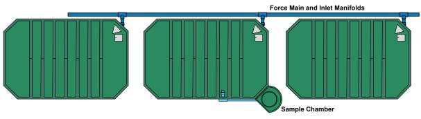
Blue coded modules with weep holes and one green coded module with sampling chamber, drain into a stone pad for final treated effluent disposal. Pad dimensions can be selected to match site conditions and modules can be installed side-by-side as well as end-to-end (as shown above)
