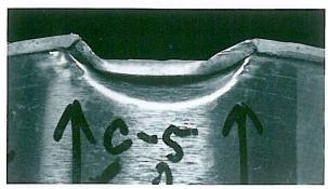
Double seam dent plate fractured.
