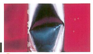
2 Severe body dent. Observe for fractured plate.
