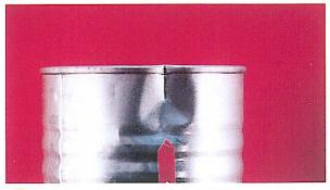
If plate is fractured in double seam or body.
