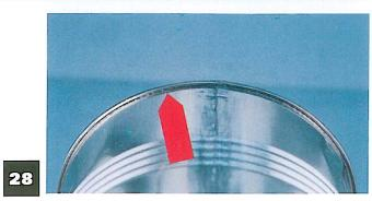
Double seam not completed-no second operation seam.
