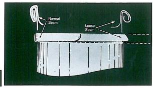
Diagram of normal and loose seam.
