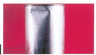
If the body dent does not significantly affect the side seam or double seam.
