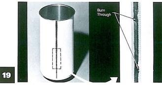
Defective welded side seam burn through.
