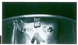
Torn flange caused by can reformer, without obvious hole.
