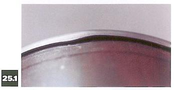
If seam thickness at bump greater than 0.003 inch with an arc dimension within 1/2–3/4 inch.
