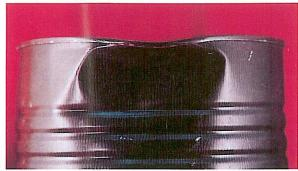
Severe body dent has affected double seam.
