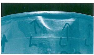
If plate fractured or opening below double seam.
