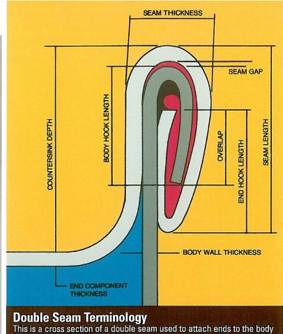
This is a cross section of a double seam used to attach ends to the body of a can. Any fracture or damage to this seam may contribute to the loss of hermetic seal and become a potential public health problem.
